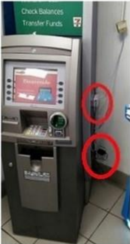
Skimmer attached to the ATM
